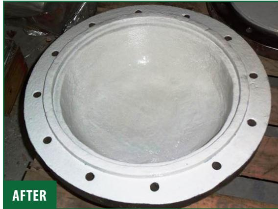
*Heat exchanger floating head before and after pits in steel were filled using **Novocoat EP3900 Machinable Paste**.
